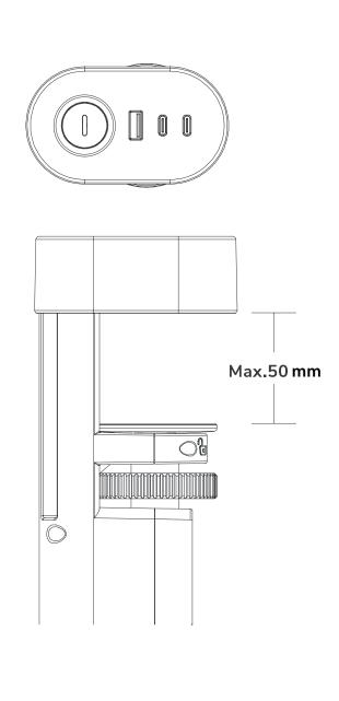
Neomounts Measuring unit: mm
